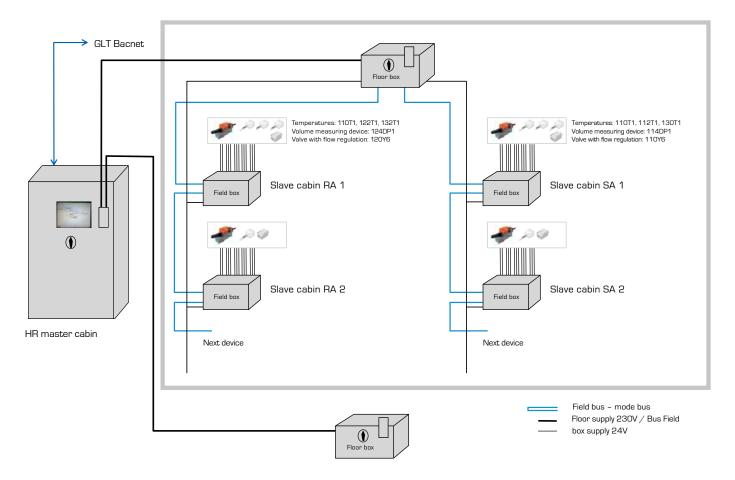
The systems are coupled to each other via a medium (circuit connected system). The number of systems that are connected in one network is determined by the use of the ventilation system (for example: conference rooms, sports halls, restauration). The common point between all the designs is a central hydraulic station per network that conveys the medium from the exhaust air to the supply air systems.
