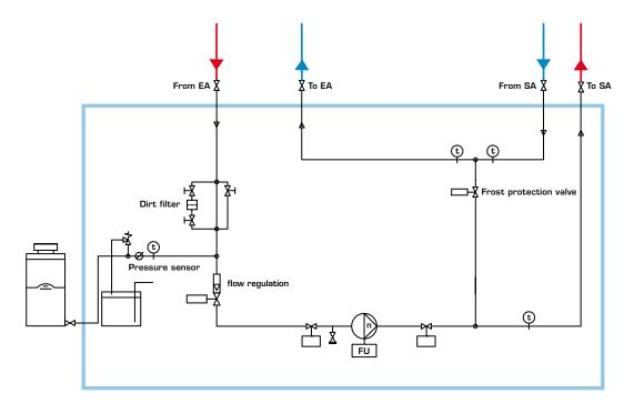
Hydraulic station with redundancy pump and heat supply
